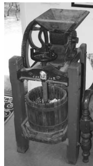
Old fashioned basket press with hand crank crusher.
