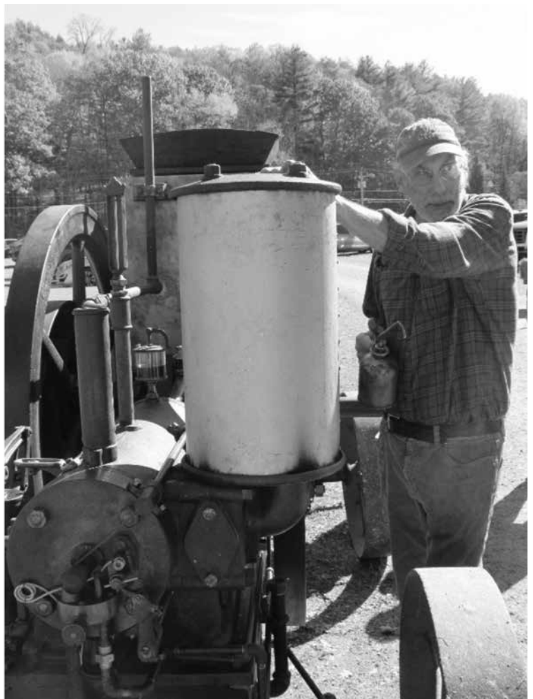
Don oils his 1900 Fairbanks Morse single cylinder gas engine at the 2019 Apple Pressing.
